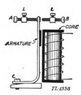
FIGURE 13 .- Voltage regulator of the generator GN-35.
